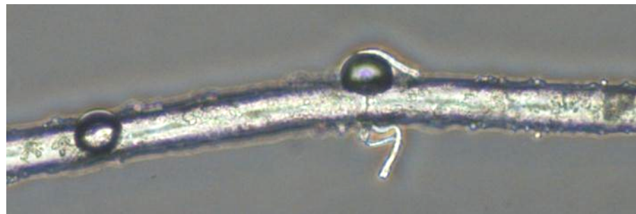
Filament covered in wax particles with abrasion damage
