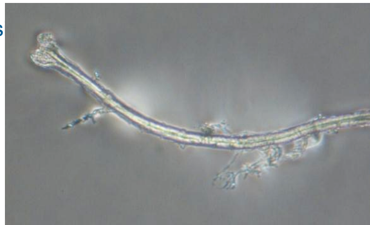
Net filament with abrasion damage from machine wash
